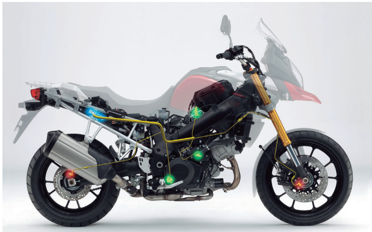
Suzuki's traction control system help riders to accelerate, brake and steer properly and efficiently, making riding safer and easier.
