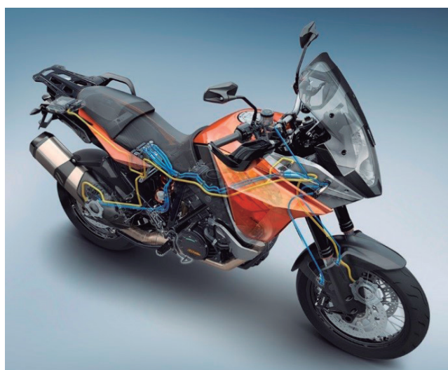
KTM has fitted its newest model with Motorcycle Stability Control, a new ABS system that allows emergency braking in curves and provides additional stability to the vehicle.
